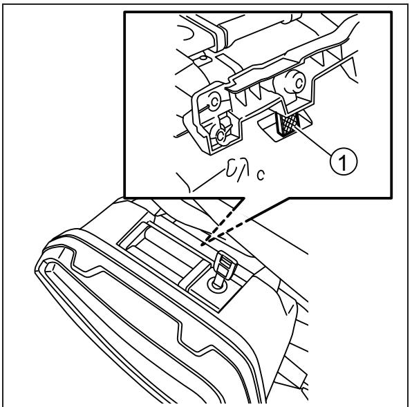
9. Hold the handle and lock lever folded down completely, then lock the case by turning the key.
