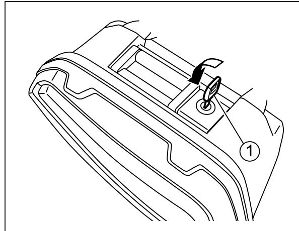
2. Lift up the lock lever ① and open the side case lid.
