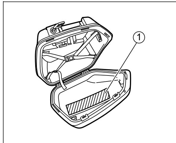
4. Secure the end of the belt ① onto the case lid.
