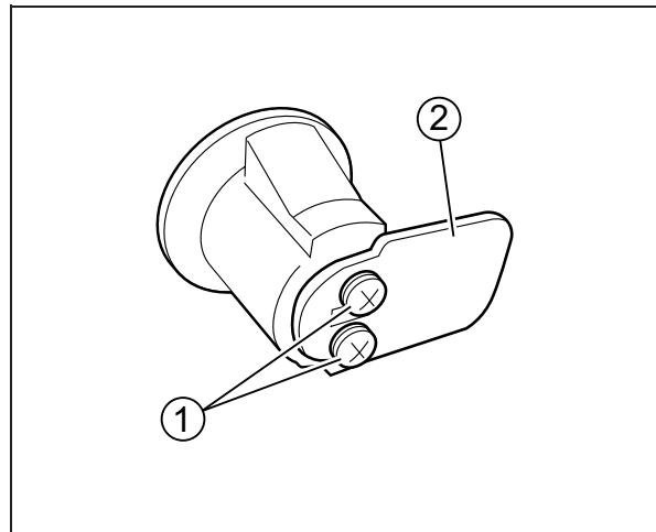
2. Insert the key cylinder into the hole ① of the side case.
